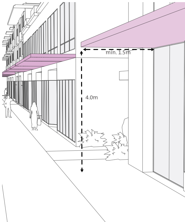
Weather protection along commercial frontages
