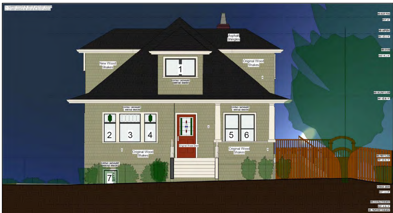
Fig. 31: Front view of Calbicks House, at 208 Fifth Avenue, 2021, highlighting the window proposal for this façade. Note the numbered windows are those that will be unchanged and preserved in-situ. (Source: D3 Dimension, Drafting and Design Inc.)
