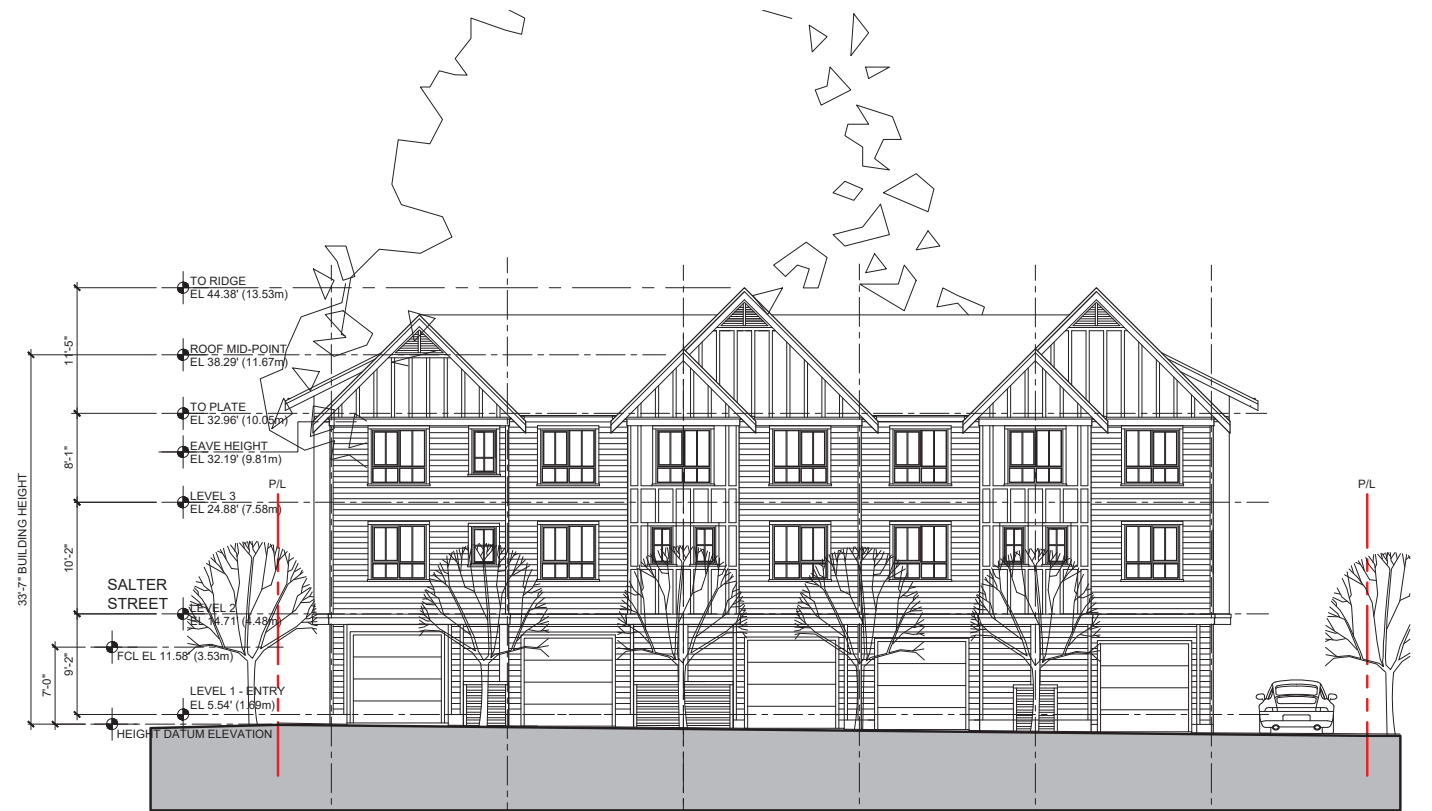
BUILDING B EAST ELEVATION 1/8"=1'-0"
