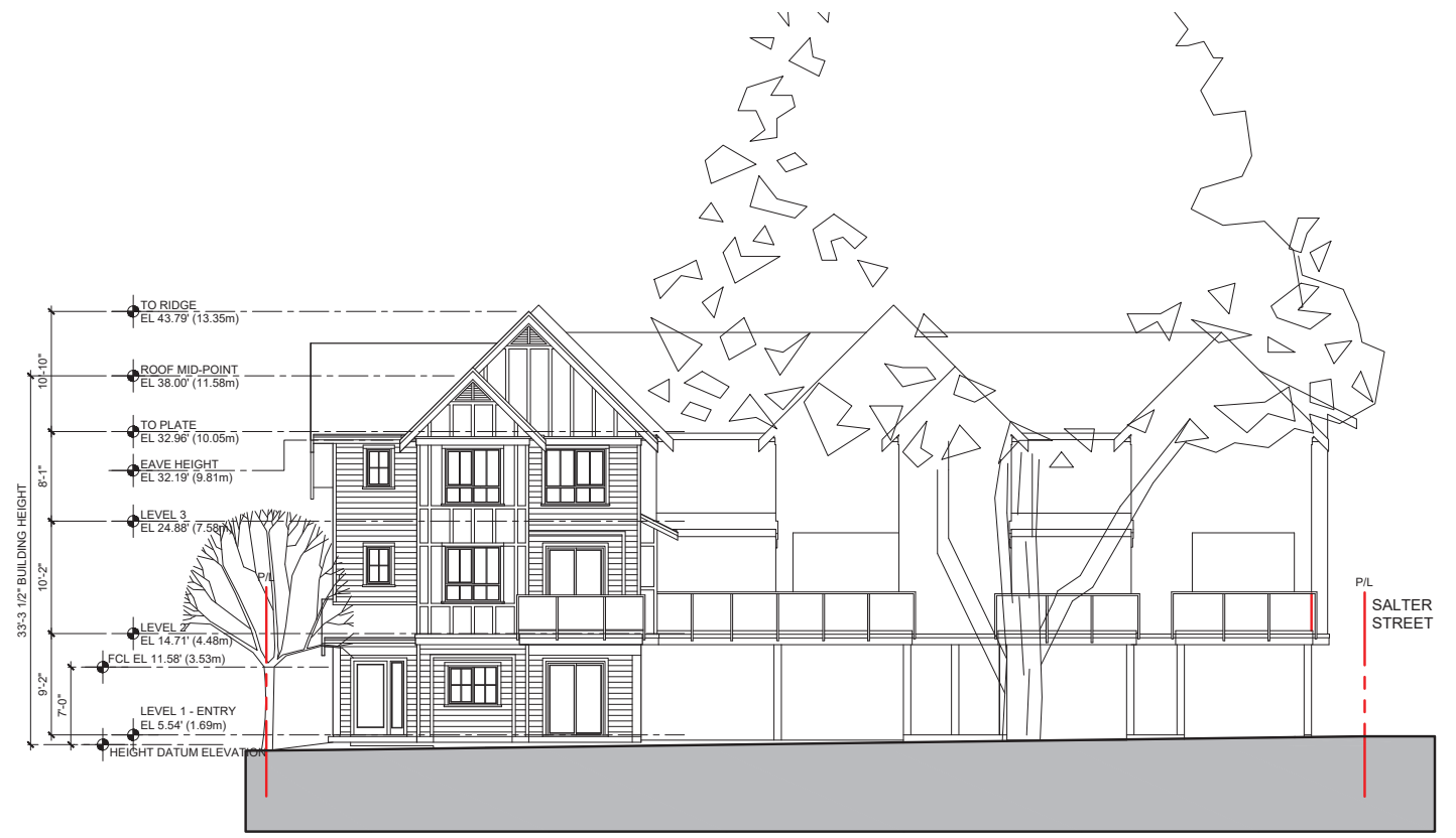
BUILDING A WEST ELEVATION 1/8"=1'-0"
