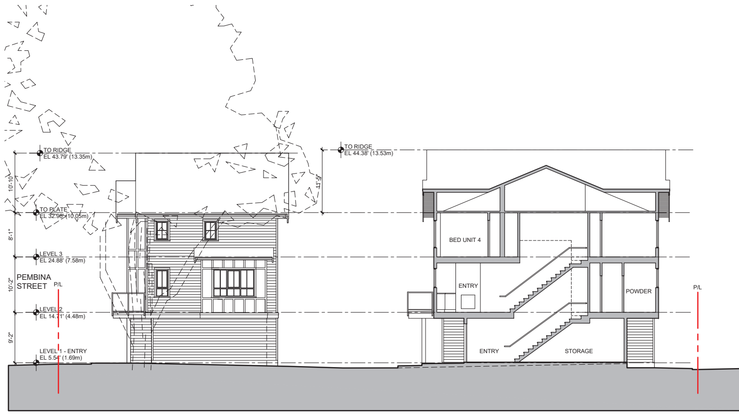
BUILDING A SOUTH ELEVATION - BUILDING B SECTION 3 1/8"=1'-0"
