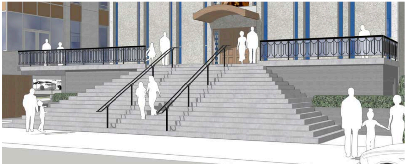
Render of proposed reconstructed and rehabilitated entrance podium and grand stair, with replicated decorative metal railing across the entire podium. Source: Surf Architecture
