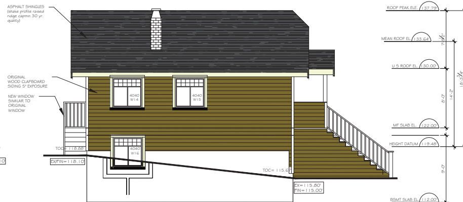
LEFT (SOUTH) ELEVATION SCALE: 1/4" = 1'-0" FACING LANE
