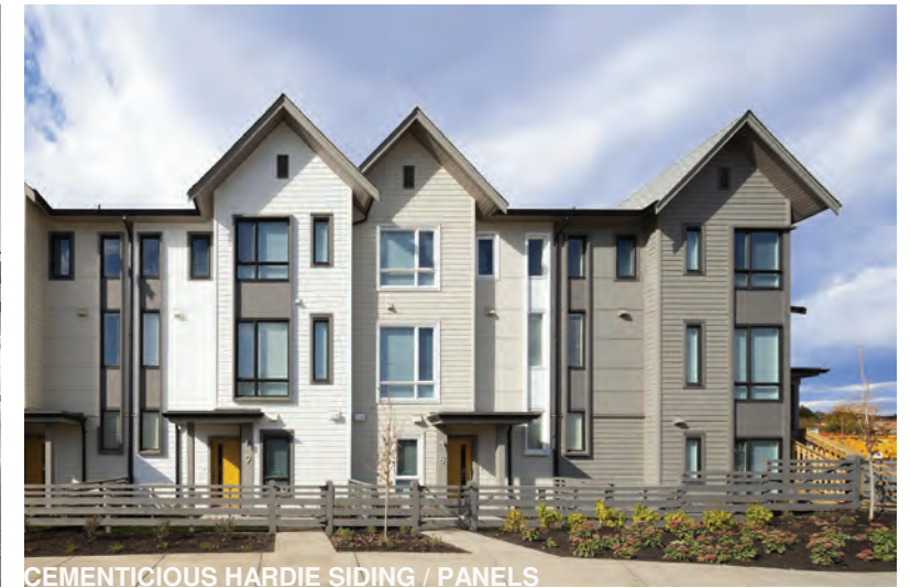
CEMENTICIOUS HARDIE SIDING / PANELS
