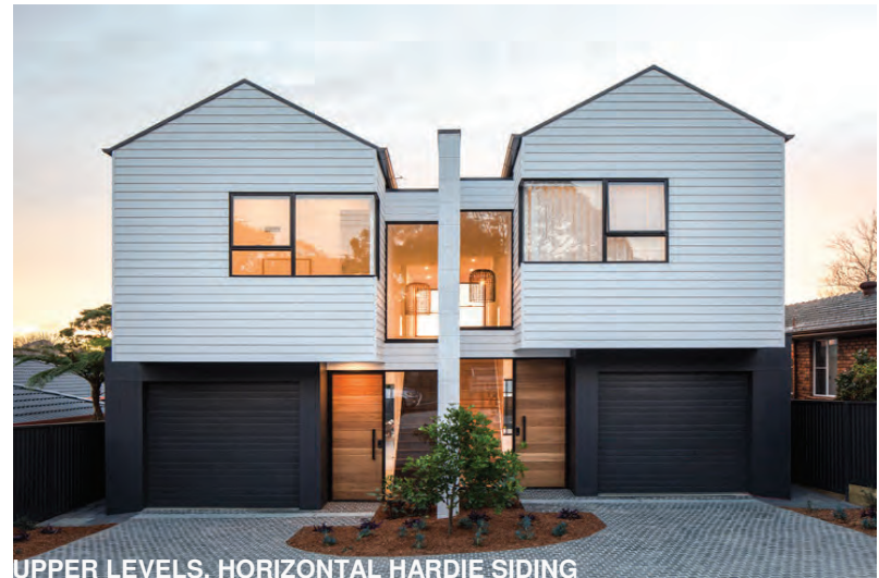
UPPER LEVELS, HORIZONTAL HARDIE SIDING
