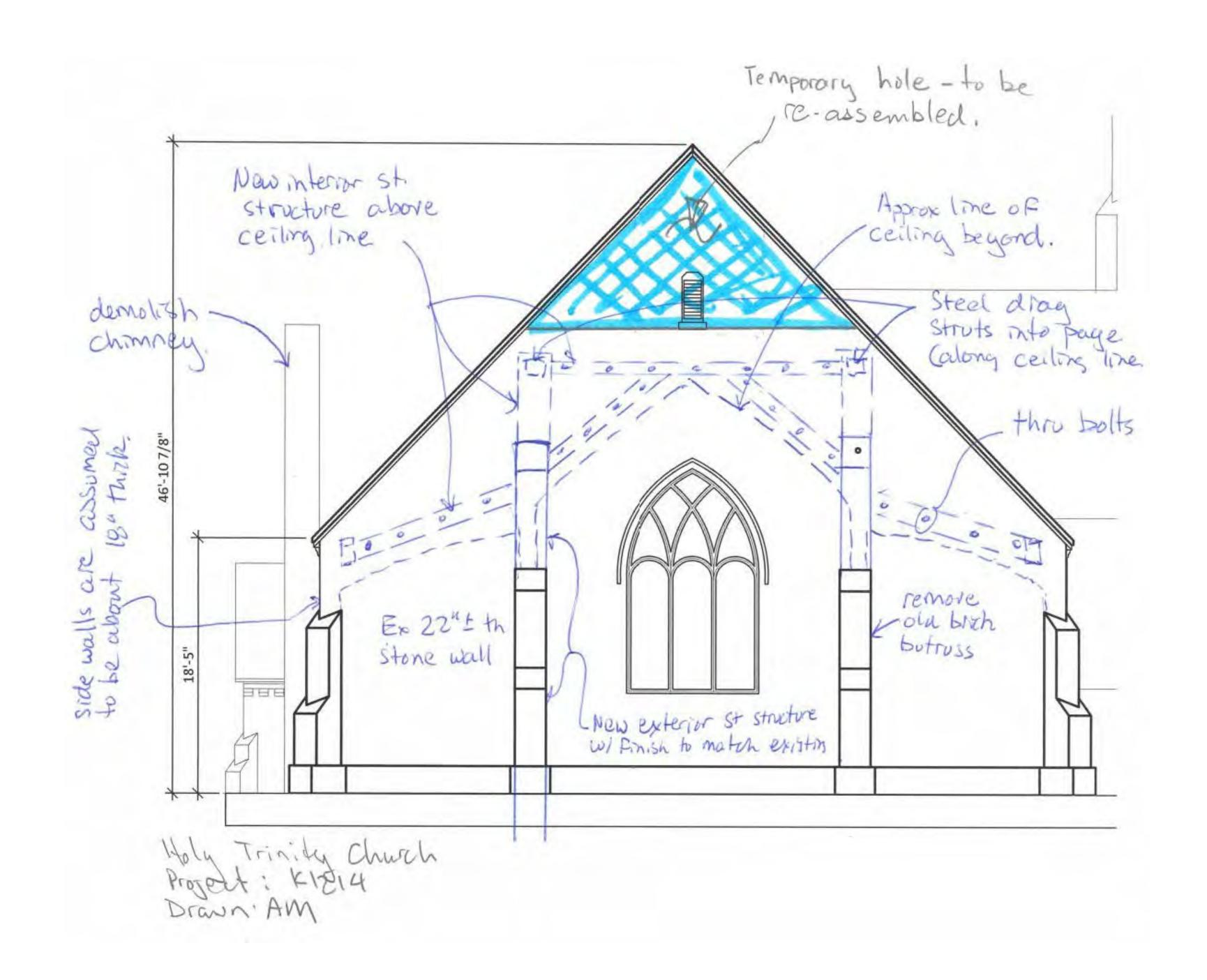
The heritage consultant team developed a less invasive approach to seismically upgrade the masonry cathedral rather than the traditional method of thickened concrete walls:
