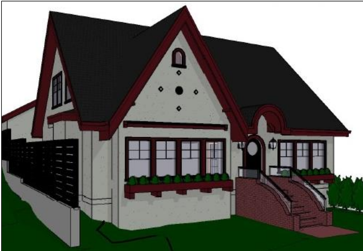
Fig. 29: Rendering of the restored front façade of Henderson House, 2020, including the restored window boxes. Note the extended height for the basement, and the resultant extended front staircase, still maintaining its brick and arched form. (Source: D3 Dimension, Drafting and Design Inc.)
