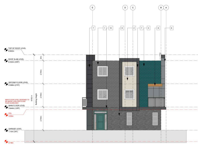
3 EAST ELEVATION Scale: 1:96
