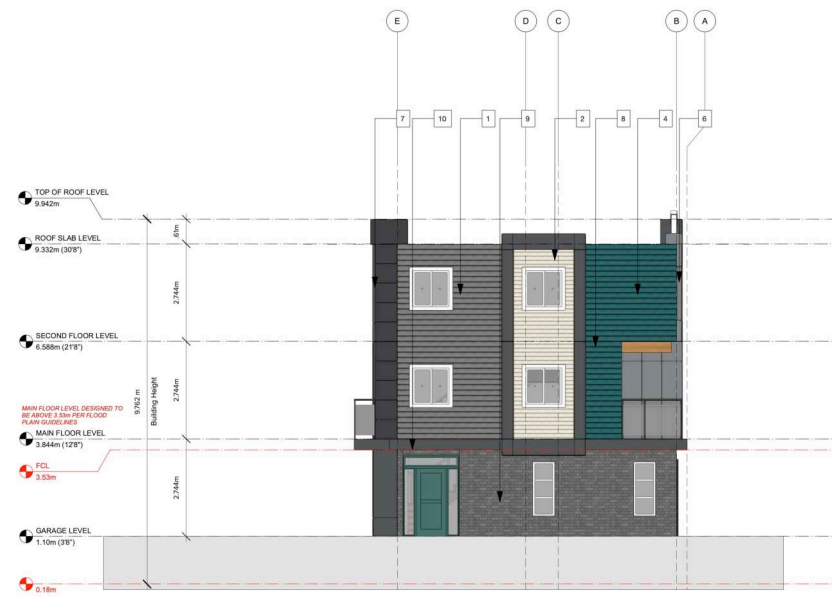
3 NORTH ELEVATION Scale: 1:96
