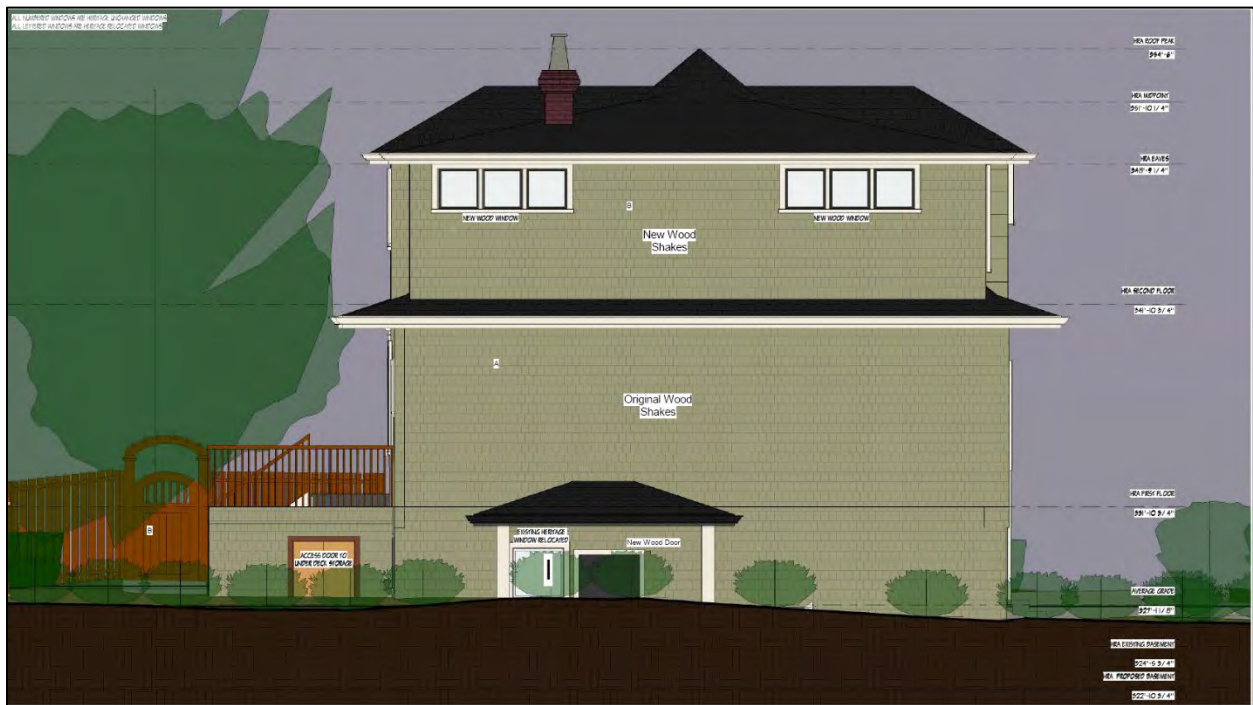
Fig. 33: Back view of Calbicks House, at 208 Fifth Avenue, 2021, highlighting the window proposal for this façade. Note the lettered windows are those that will be preserved, but relocated. (Source: D3 Dimension, Drafting and Design Inc.)
