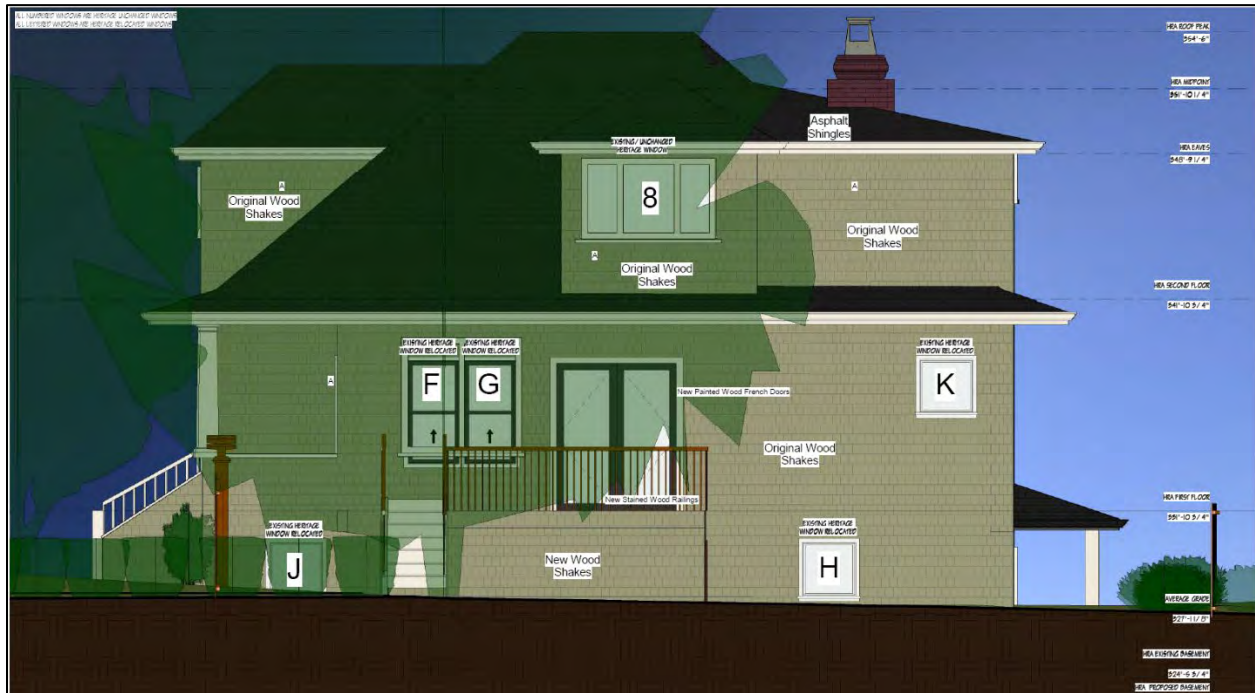
Fig. 34: Western side view of Calbicks House, at 208 Fifth Avenue, 2021, highlighting the window proposal for this façade. Note the numbered windows are those that will be unchanged and preserved in-situ and the lettered windows are those that will be preserved, but relocated. (Source: D3 Dimension, Drafting and Design Inc.)
