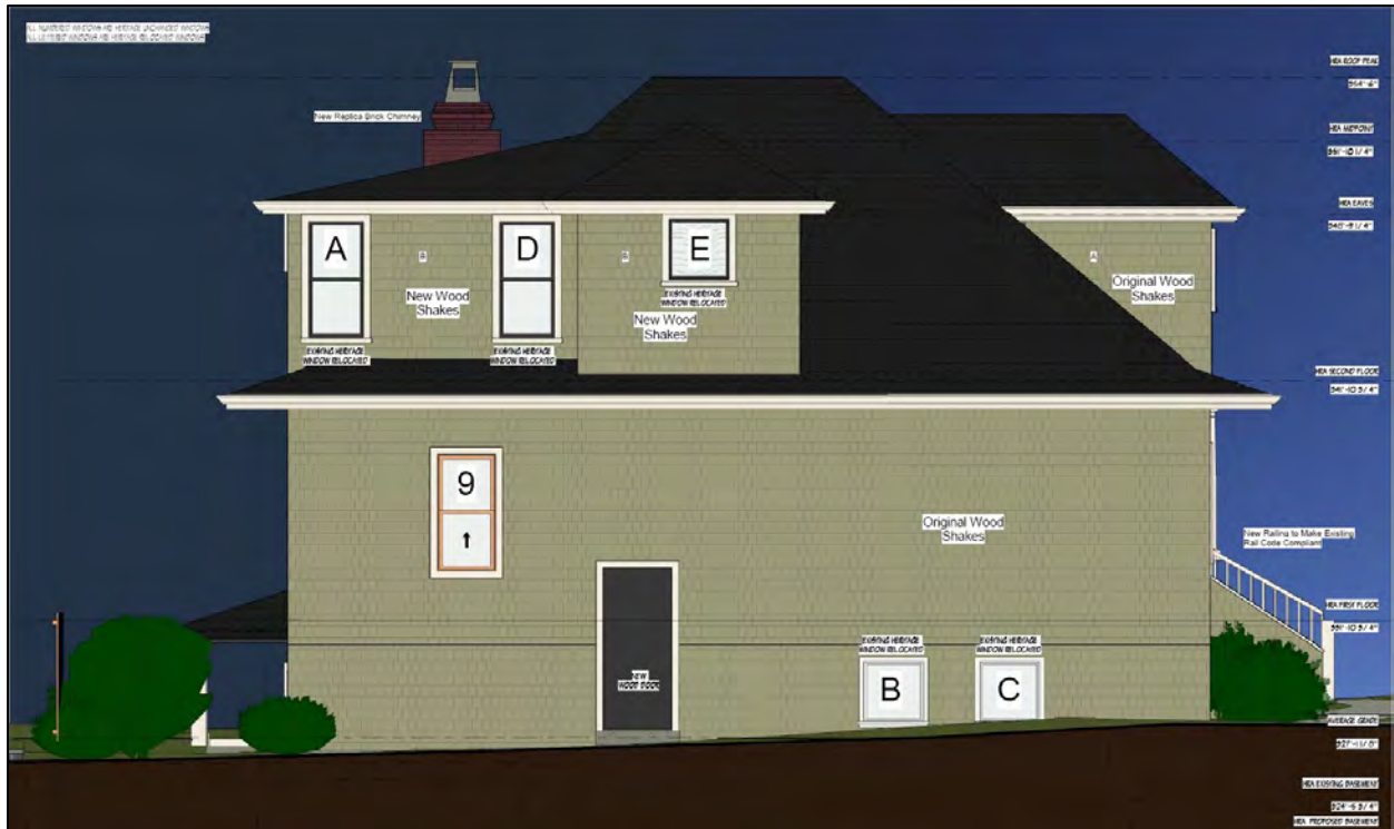
Fig. 32: Eastern side view of Calbicks House, at 208 Fifth Avenue, 2021, highlighting the window proposal for this façade. Note the lettered windows are those that will be preserved, but relocated. (Source: D3 Dimension, Drafting and Design Inc.)
